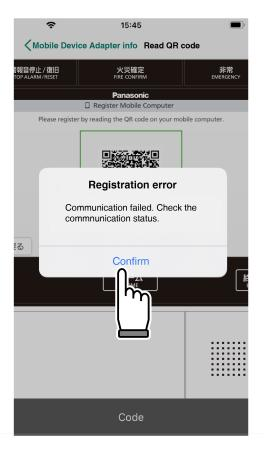
Confirm that the LAN cable is connected, and the wireless LAN communication stat us is normal.
